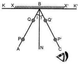
Fix two steel pins P and Q on the straight line AB atleast 10 cm apart. Look for the images of the pins P and Q and fix two pins P Q' such that P', Q' and images of P and Q are all in the same straight line. Remove the pins and draw small circles around the pin pricks.
